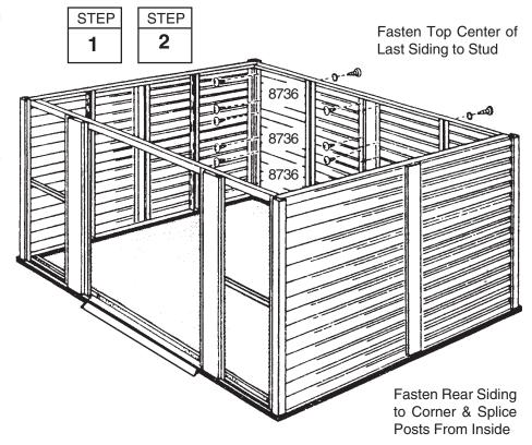
${f 3}$  Slide **front siding** into channels of corner post and door jamb. This siding is fastened from the inside, using screws into post and jamb.
