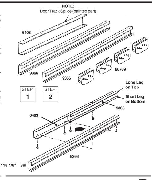
Position door slides onto the legs, from the end of door track assembly, as shown in the end view.
