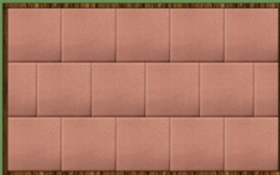
Fig shows tiles laid brick-bond with timber edge restraint
