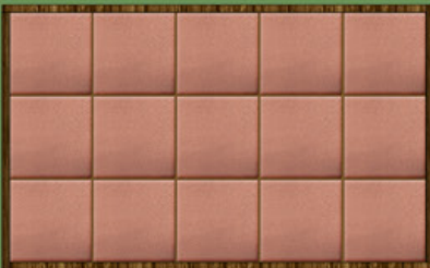
Fig shows tiles laid in a grid pattern with timber edge restraint
